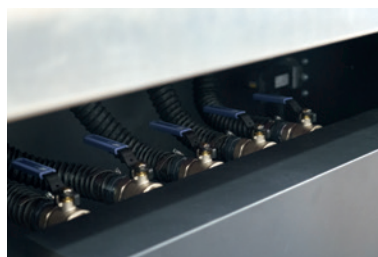
Vacuum sectioned throughout the equipment for more efficient and controlled media transport.
