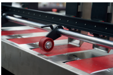
All cardboard feeding is controlled by crush wheels, controlling thickness and avoiding material vibrations.
